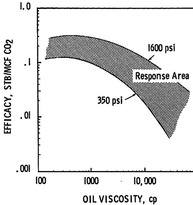
Fig. 4 - **CO<sub>2</sub> STIMULATION DOES NOT REQUIRE HIGH OIL SATURATION**
