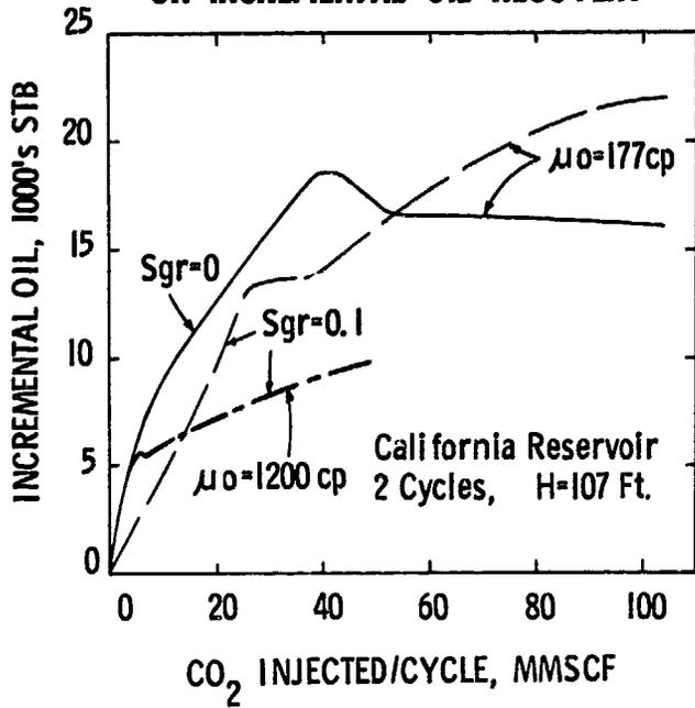
Fig. 2 - CO<sub>2</sub> HUF-n-PUF PROCESS BOTTOM HOLE PRESSURE EFFECT
