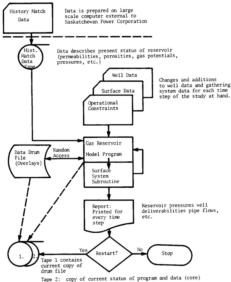
Fig. 10 - Gas reservoir management program, system flow chart.
