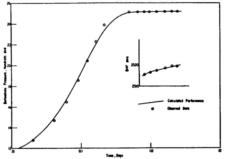
Fig. 2 - Field Application #1 Pressure Buildup Test
