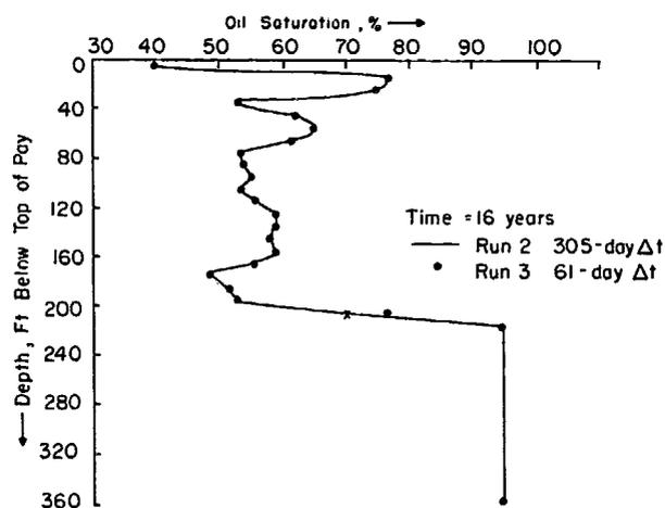
FIG. 6 — COMPARISON OF OIL SATURATION DISTRIBUTIONS FROM ONE-DIMENSIONAL CALCULATIONS.
