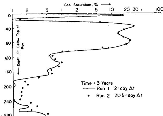
FIG. 4 — COMPARISON OF GAS SATURATION DISTRIBUTIONS FROM ONE-DIMENSIONAL CALCULATIONS.
