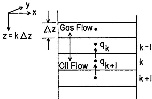
FIG. 1 — UPWARD GAS FLOW IN A COLUMN OF BLOCKS.
