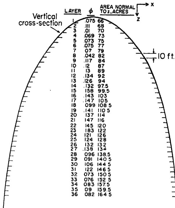
FIG. 2—POROSITY AND CROSS-SECTIONAL AREA OF A PINNACLE REEF.
