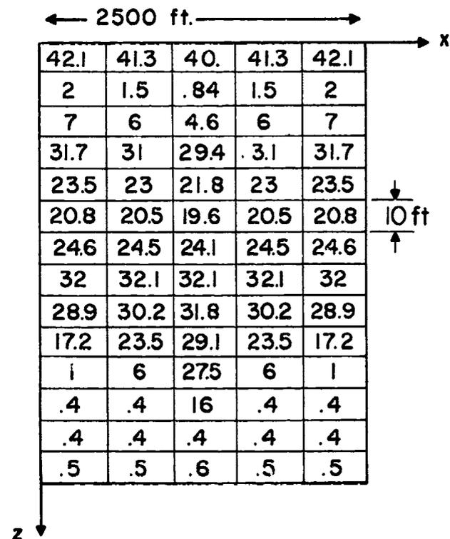
FIG. 7 — GAS SATURATION DISTRIBUTION AT 5 YEARS, FROM TWO-DIMENSIONAL CALCULATION.
