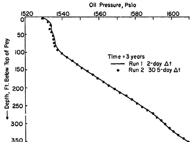
FIG. 5 — COMPARISON OF OIL PRESSURE DISTRIBUTIONS FROM ONE-DIMENSIONAL CALCULATIONS.
