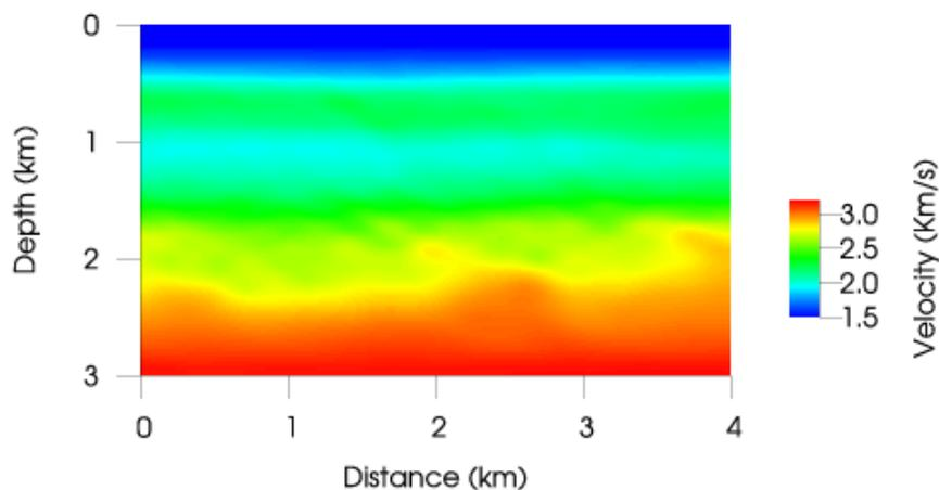
**Figure 4** Velocity model estimated with full-waveform inversion in the image space using the model in Figure 1 as the initial velocity field.
