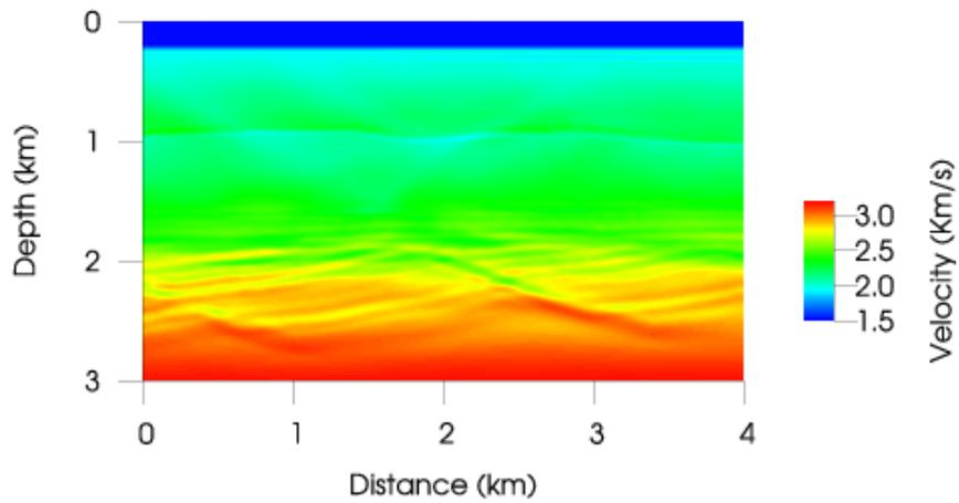
**Figure 2** Velocity model estimated with full-waveform inversion in the data space using the model in Figure 1 as the initial velocity field. Note the discrepancy with the true model shown in Figure 3.
