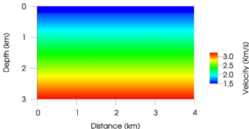
**Figure 1** One-dimensional initial model with linear velocity increase.
